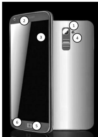
Fig. 7: Potential VCSEL based sensors in a Smartphone. (1) Autofocus, (2) Proximity, (3) + (4) video signal to display and from camera, (5) low noise microphone, (6) gesture recognition
