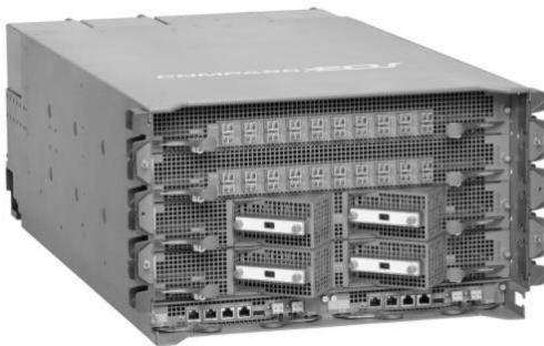
Fig. 2: The r10004 core router by Compass EOS is unique in compactness and power consumption while offering 1.34 Tbps aggregate bandwidth (Source: Compass EOS)
